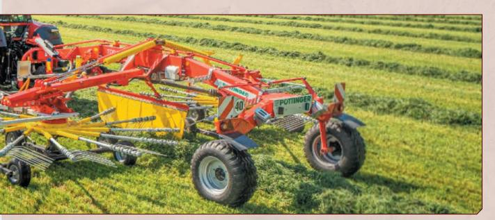
Replacing the rotor chassis wheels, this glide bar offers the best reliability in challenging ground conditions. Flowtast glides effortlessly over even deep ruts, holes, and wheel marks. The glide bar is especially suitable for soft and damp soil conditions.
