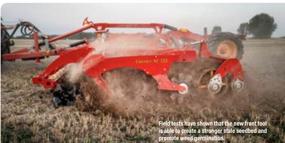
A new front tool option is now available for ultra-shallow tillage and mechanical weed control.
